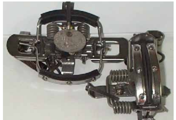
Jaw traps for rabbits, cats, foxes and dogs must by law have rubber-covered, soft jaws. You can use old leaf sprung rabbit traps that have been upgraded or buy these coil sprung coyote-type traps.
