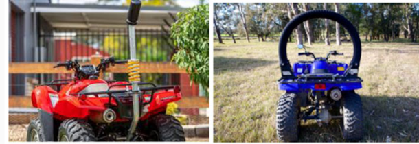
Examples of Operator Protective Devices for Quad Bikes
