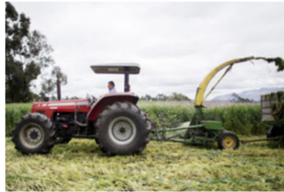
Example of rollover protection on a tractor
